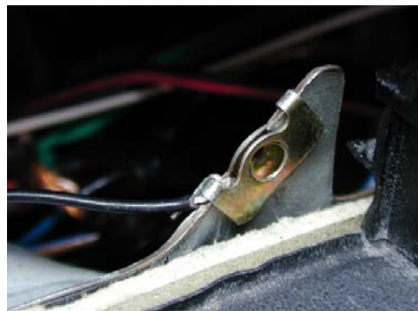
Find a ground point for the black wire.
