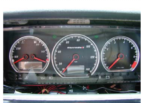
Reinstall the instrument cluster. Connect the 3 harnesses from the gauges to the harness on the inverter. There is an extra harness (on the inverter) for the oil/volt gauges (late 1993 and up models).
