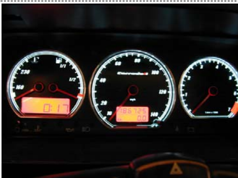
Turn the ignition to the ON position. Gauges should illuminate. If not, please check FAQ. Adjust the brightness with the dimmer. Reinstall the cluster front cover.
